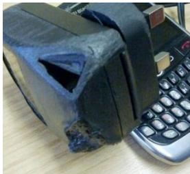
If any signs of damage are found, the equipment must not be used. These simple user checks do not need to be recorded.
