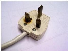
Inspect for obvious damage to the cover(s) of the equipment.
