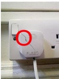
Inspect the cable for damage.
